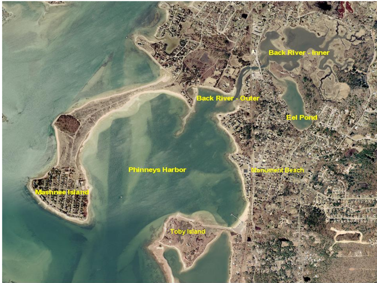
Figure I-1 Phinneys Harbor (inclusive of Eel Pond and Back River) study region for the Massachusetts Estuaries Project nutrient analysis. Tidal waters enter the estuarine system through one inlet to Buzzards Bay. Freshwaters enter from the watershed primarily through 1 surface water discharge (stream from Mill Pond to Back River upgradient of County Road) and direct groundwater discharge.
