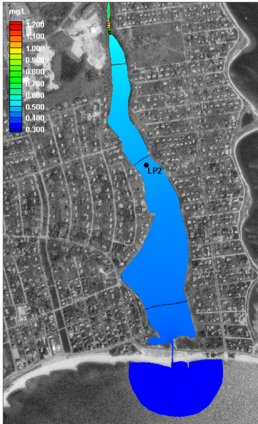
Figure VIII-1. Contour plot of modeled average total nitrogen concentrations (mg/L) in the Little Pond system, for threshold conditions (0.45 mg/L at water quality monitoring station LP2). The approximate location of the sentinel threshold station for Little Pond (LP2) is shown.
